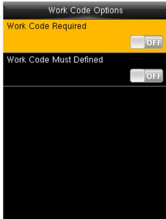
**Work Code Required:** The work code must be input during verification. Select whether to enable this function.
