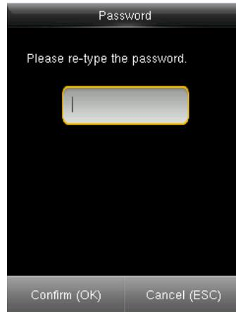
Input 1-8 digits password and press [M/OK], then rewrite the password.
