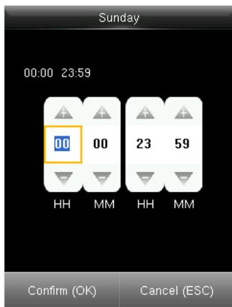
If the end time is in advance than the start time, for instance: 23:57- 23:56 , the whole day is forbidden to open the door. If end time is after than start time 00:00- 23:59 , it is effective section. Effective time zone for user unlocking: 00:00-23:59 or end time is bigger than start time. Note: The default time period number 1 indicates all-time access (that is, newly registered users are unlocked).
