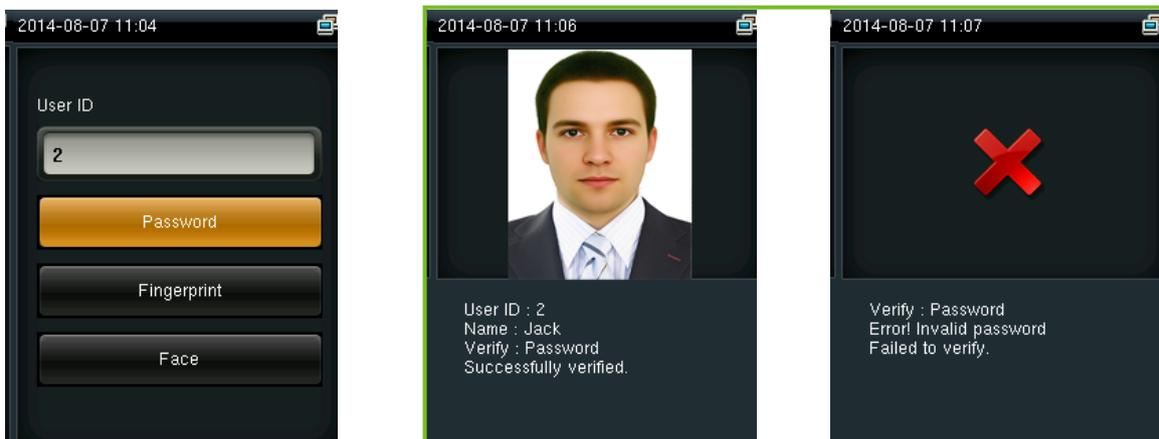
Note: The device says *"Incorrect password"* when failed to verify. You can try another 2 times. If it fails after 3 times, return to the initial interface.
