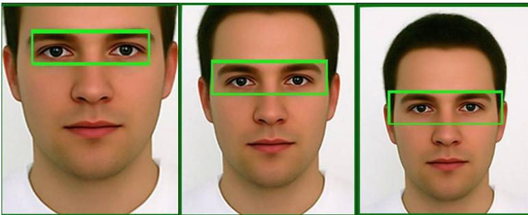
During enrollment, locating your face appears in the center of the screen, and follow the voice prompts "Focus eyes inside the green box". The user needs to move forward and backward to adjust the eyes position during the face registration.
