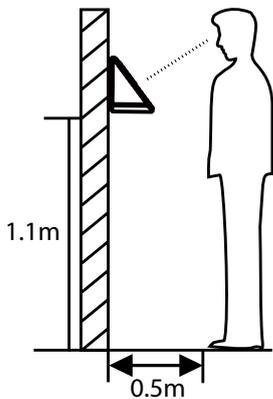
For users 5-6 feet tall (1.55m-1.85m), we recommend users stand about 2 feet (0.5m) from the device. When viewing your image on the device display window, step away if your image appears too bright. Step closer if your image appears too dark.
